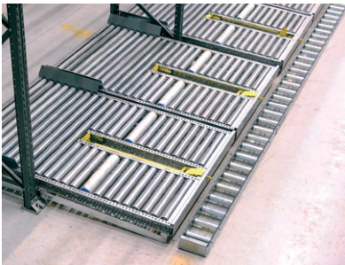
Front roller track for moving of empty pallets
