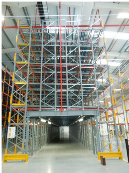
Pallet live installation with picking tunnel
